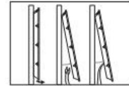
(3) Pull down two strings together to unlock the brackets from the wall plate, then you can take brackets down.
