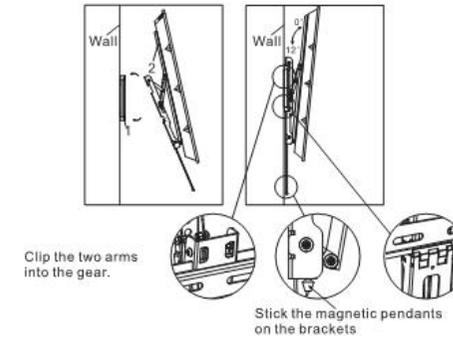
(1) Press the brackets after you put them on the wall plate, then they would be locked with wall plate.
